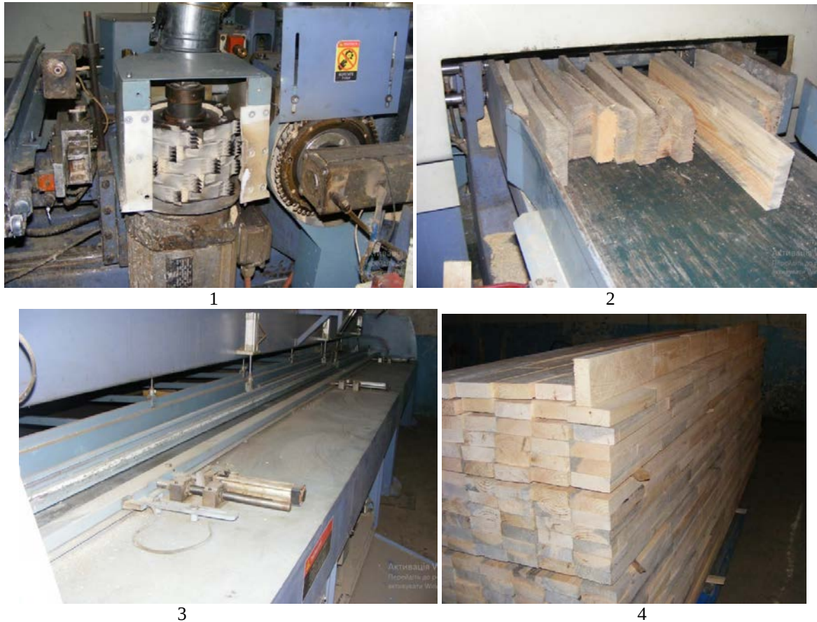
Fig. 5. Production of the finger joined glulam: 1 – machinery with shaper knives, 2 – cut semi fabrications before finger-joining, 3 – press machine of finger joint line, 4 – glulam.
