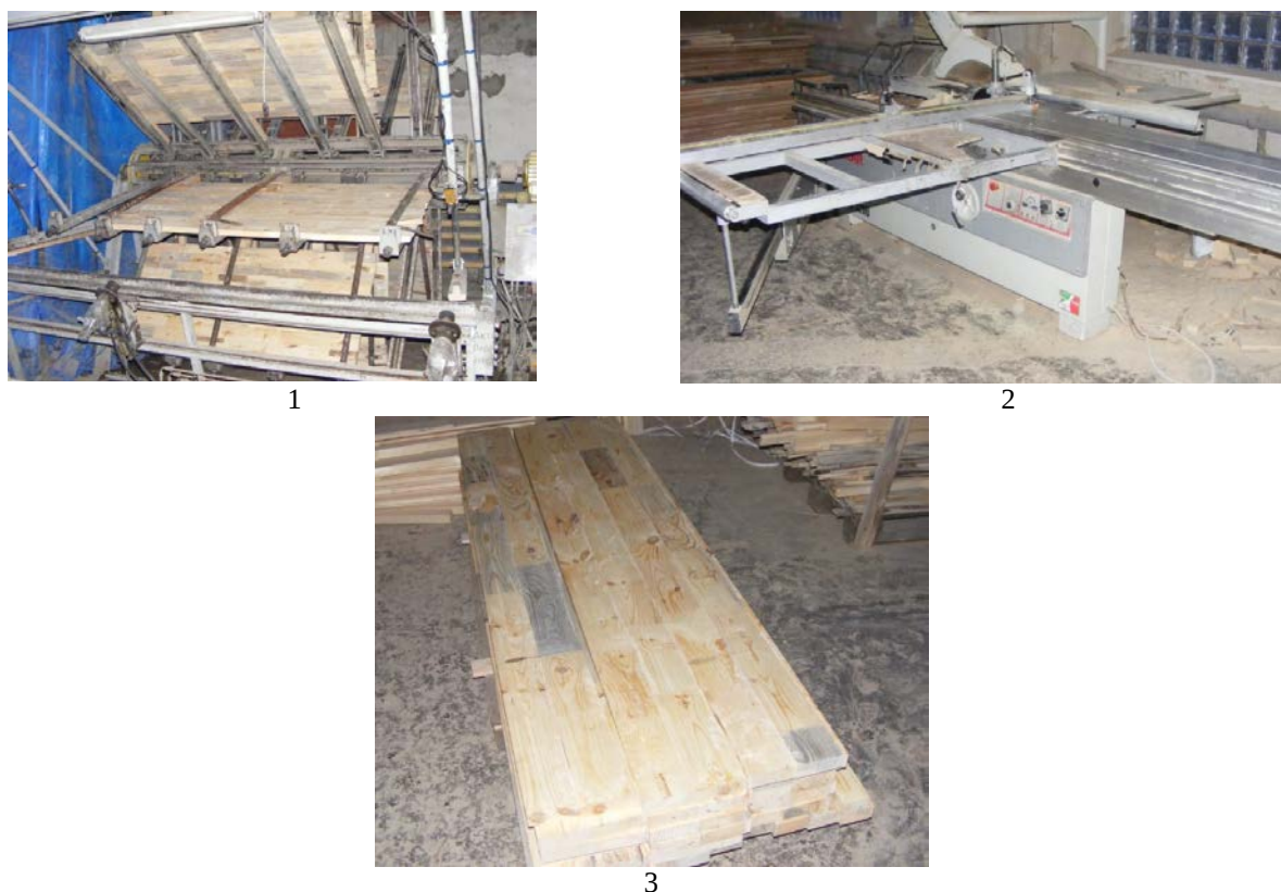
Fig. 7. Production of the furniture boards: 1 – press machine for transverse gluing, 2 – panel-sizing machine SICAR BOOM-3200, 3 – formatted furniture boards.
