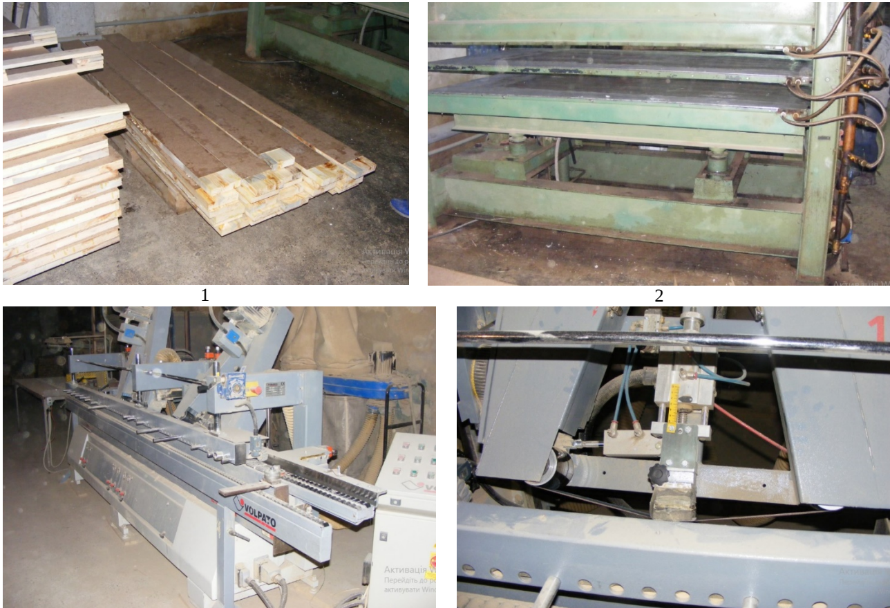
Fig. 9. Covering of parts by veneer: 1 – wooden beams covered by MDF, 2 – press machine used to cover beams and frames by MDF, 3 – Grinding machine for wooden beams.
