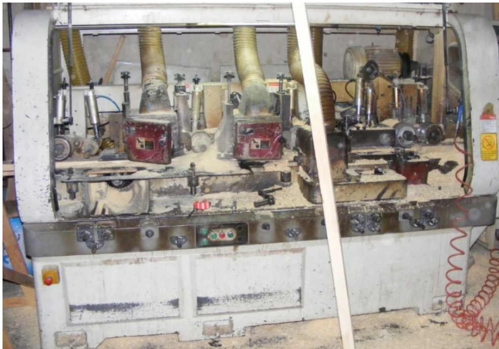
Fig. 6. Wood wool on the four-sided machine after profiling of the glulam.
